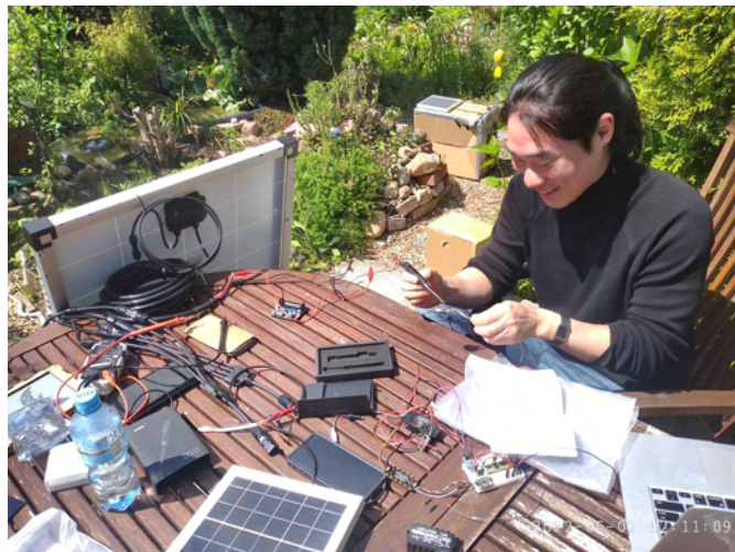
Abb. 4: Experiments with solar soldering in the garden colony "Dreieck Nord off-the-grid and without battery.
